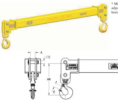
\* Minimum horizontal top rigging angle is 45° on all fixed and adjustable spreaders. M&W recommends a minimum horizontal top rigging angle of 60°.
