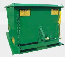
Safety retaining chain and trip rope store conveniently on the back of the unit when not in use.
