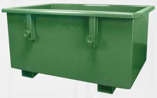
Extra heavy duty container fabricated from 3/8" plate. Designed for transport with overhead crane and to be emptied with rollover attachment on forklift. Used by bearing manufacturer.
