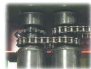
OPTIONAL 3" RC NOW AVAILABLE (guard removed for clarity)
